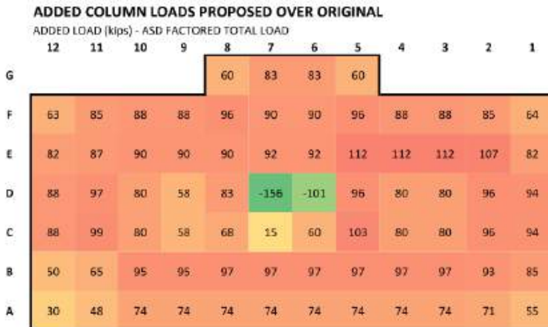
Figure 10: Added Column Loads – Proposed over Original
